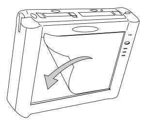
Figure 3. Installing the Screen Protector
